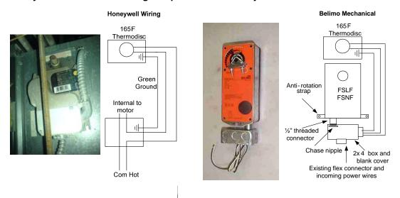
If necessary add a chase nipple and junction box as shown above right for wiring connections.
