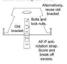
In all cases, the stud of the anti-rotation strap should fit in the middle of the slot at the bottom of the Belimo. This allows the actuator to move as necessary to compensate for any non-concentric rotation of the damper shaft.
