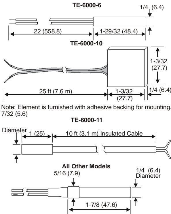
Note: Element is furnished with adhesive backing for mounting.
