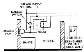
Fig. 3 — Typical wiring diagram of Humidistat to control humidity in homes during heating season by automatic control of exhaust fan.
